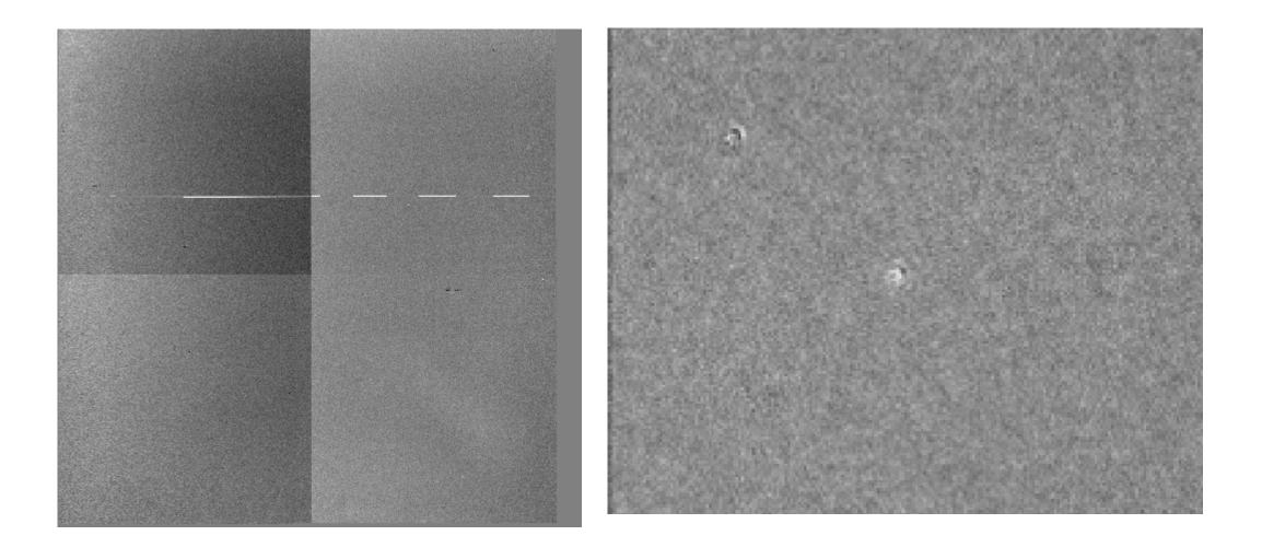
• Aperture Photometry (Sextractor): Aperture photometry involves aligning a selected aperture size with the point source to be measured, counting the total number of photons within the aperture, and then subtracting the number of background photons to obtain the flux of the point source. Subsequently, the instrumental magnitude is calculated based on this flux.
