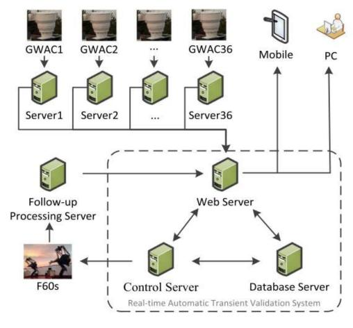
System Architecture and data processing stream. The RAVS is in the dashed-line box. The data flow is shown by the arrows.
